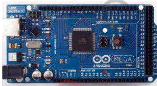
Gambar 1.7 Arduino Mega 2560
