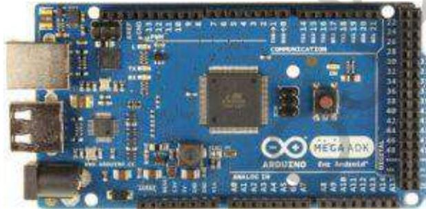
Gambar 1.12 Arduino Mega ADK
