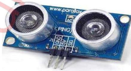
Gambar 1. Sensor Ultrasonik PING
