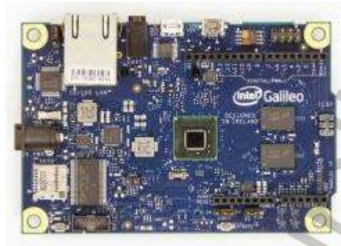
Gambar 1.8 Arduino Intel Galileo
